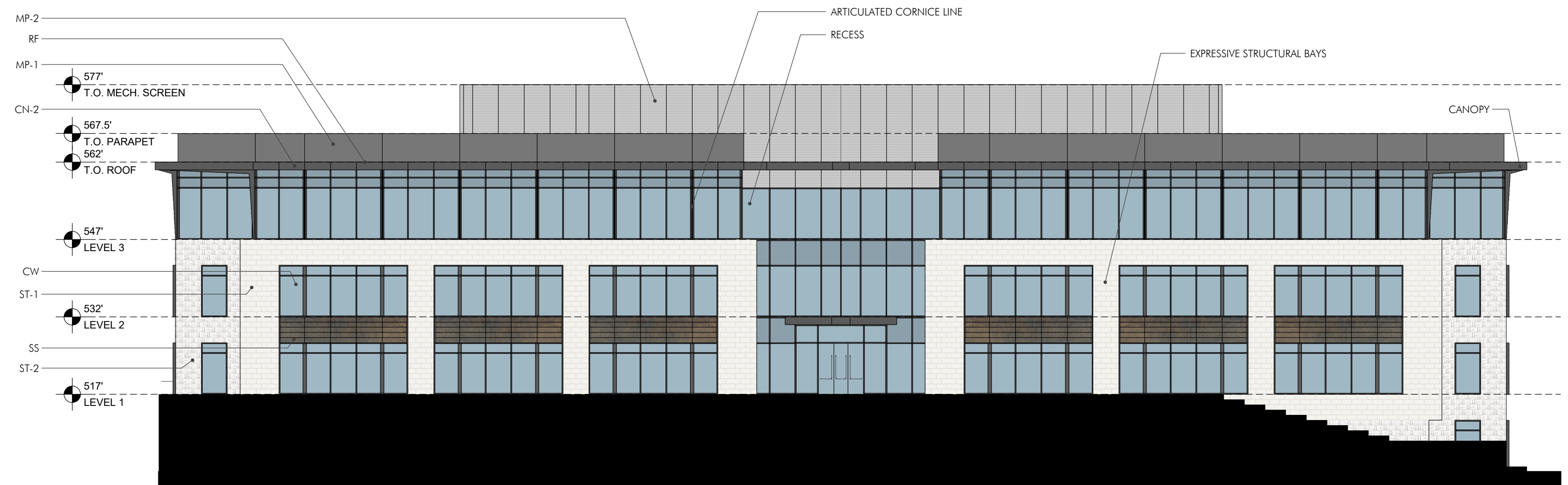
2 SOUTH ELEVATION BUILDING STRUCTURE Scale: 1/16" = 1'
