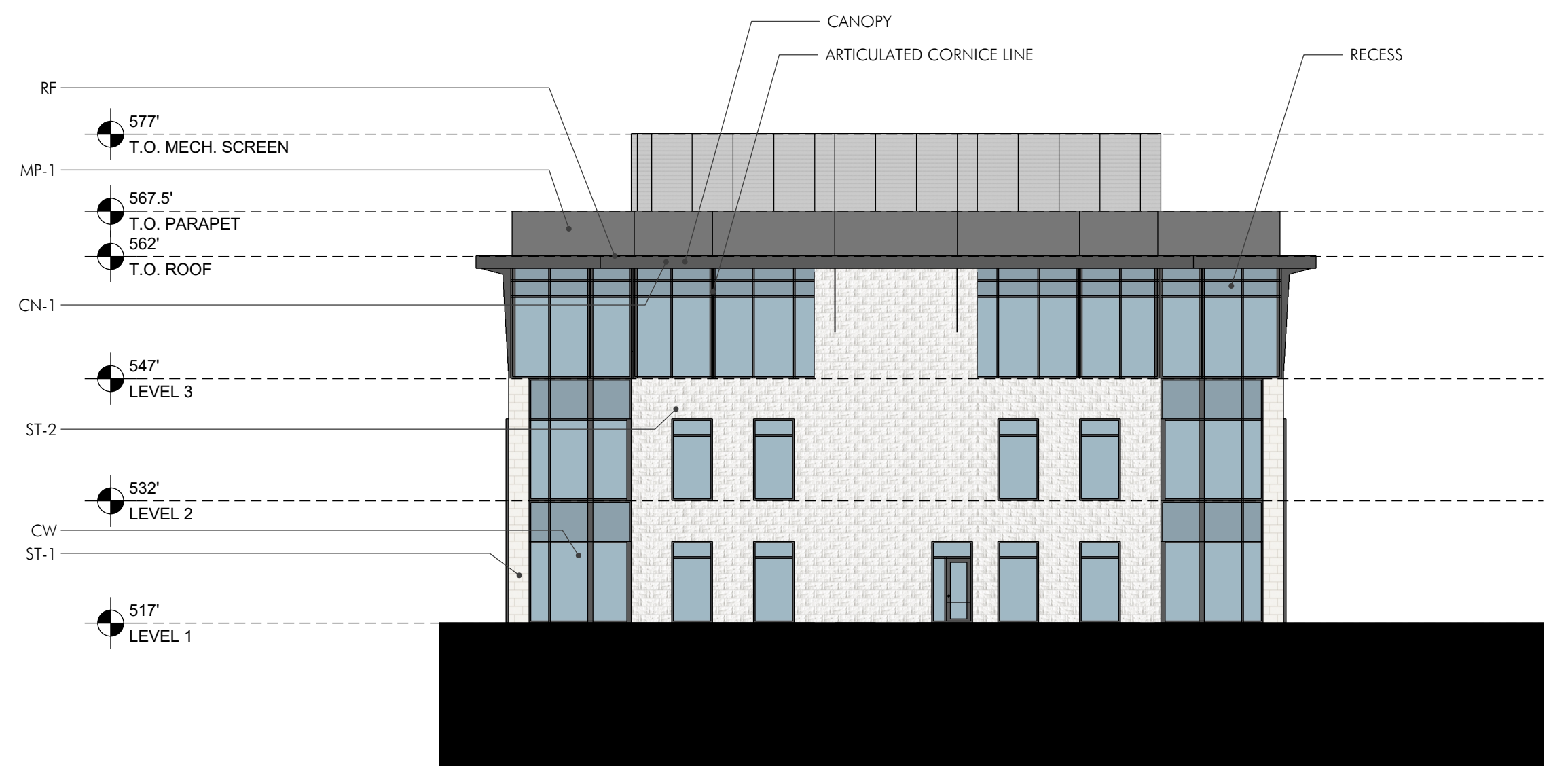
4 WEST ELEVATION BUILDING STRUCTURE Scale: 1/16" = 1'
